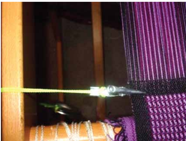
Temple in use on left side of loom. The weight is suspended over the side bar.
