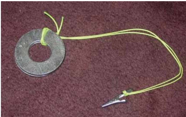
Temple with washers for weights and alligator (croc) clip to attach to the cloth
